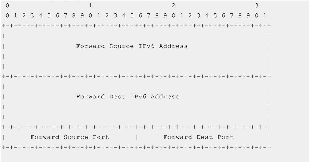
Figure 21 : Binary Logging Format - forward tuple: IPv4 in IPv6
