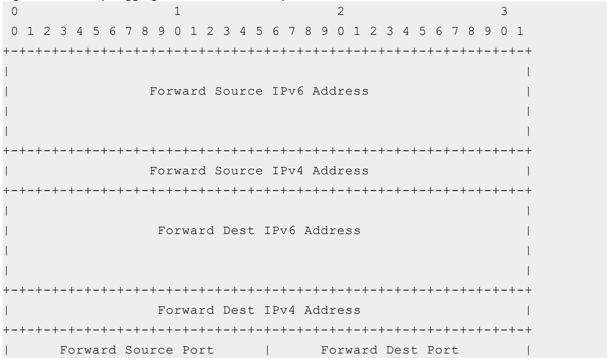
Figure 21 : Binary Logging Format - forward tuple: IPv4 in IPv6
