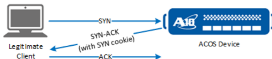
Figure 25 : SYN-ACK Handshake (Legitimate Client)
