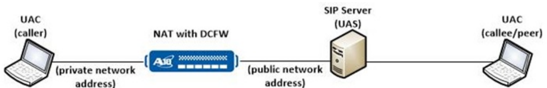
Figure 6 : Network Topology diagram for NAT with firewall for SIP traffic
