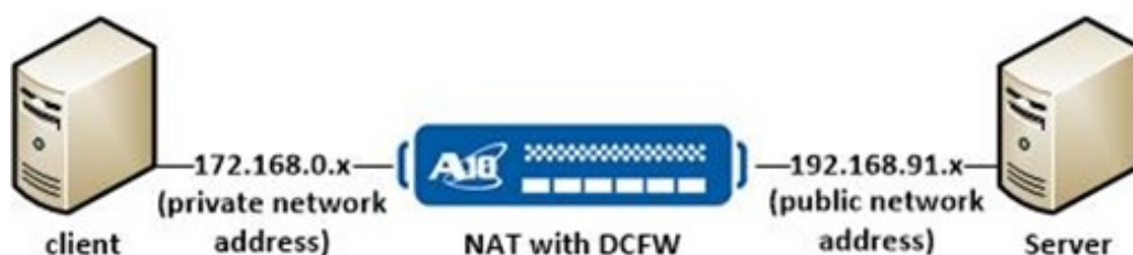
Figure 4 : Network topology diagram for NAT with firewall
