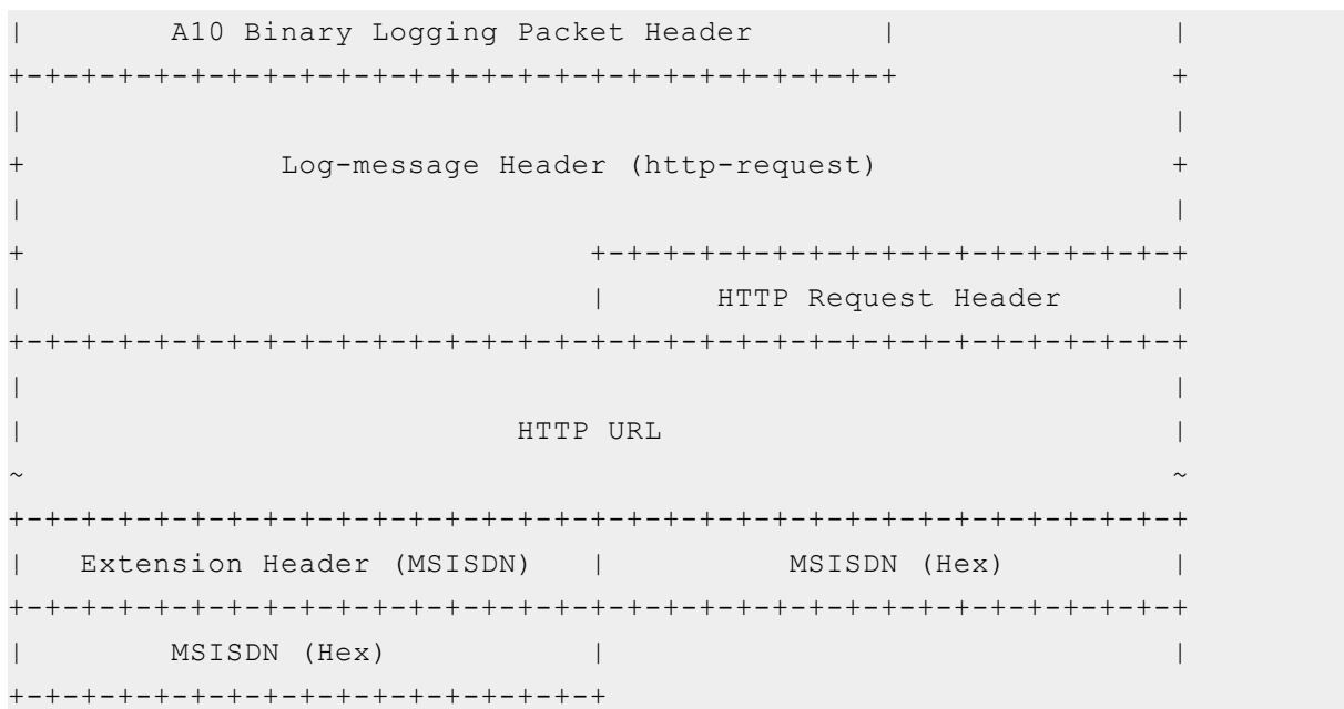
Figure 59 : Binary Logging Format - include client mobile number (MSISDN), HTTP request information including hostname, HTTP method, and Layer 4 session information
