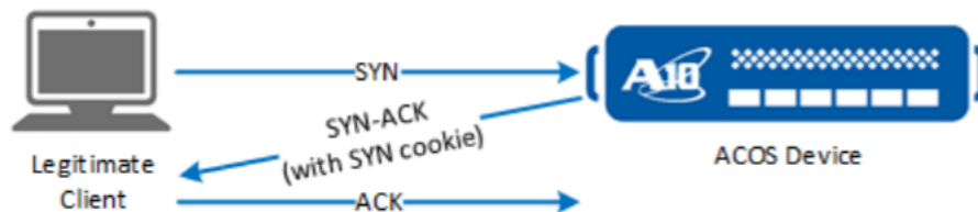
Figure 25 : SYN-ACK Handshake (Legitimate Client)
