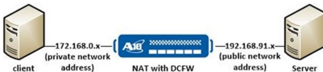
Figure 4 : Network topology diagram for NAT with firewall
