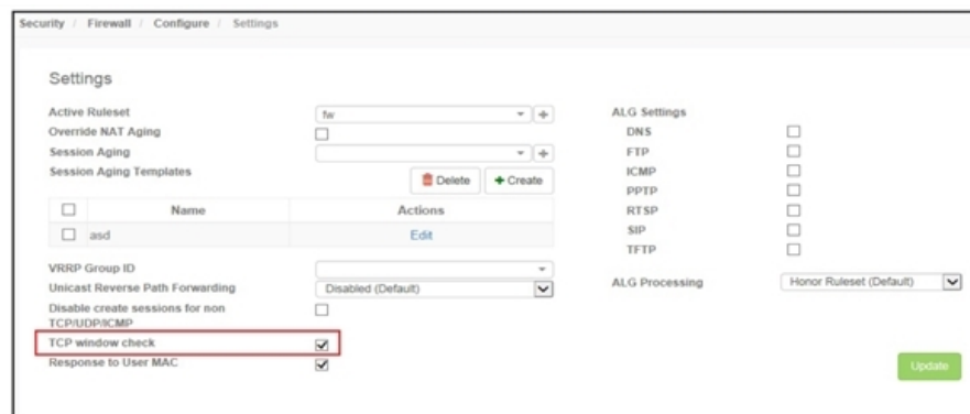
Figure 8 : Configuring TCP Window Checks using the GUI
