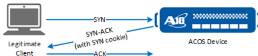
Figure 25 : SYN-ACK Handshake (Legitimate Client)
